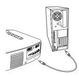
Connect the other end of the audio cable to the speaker or audio out port on the computer's sound card. If you don't need to make any other connections, you can plug in and turn on your equipment; see page 23 for instructions.
